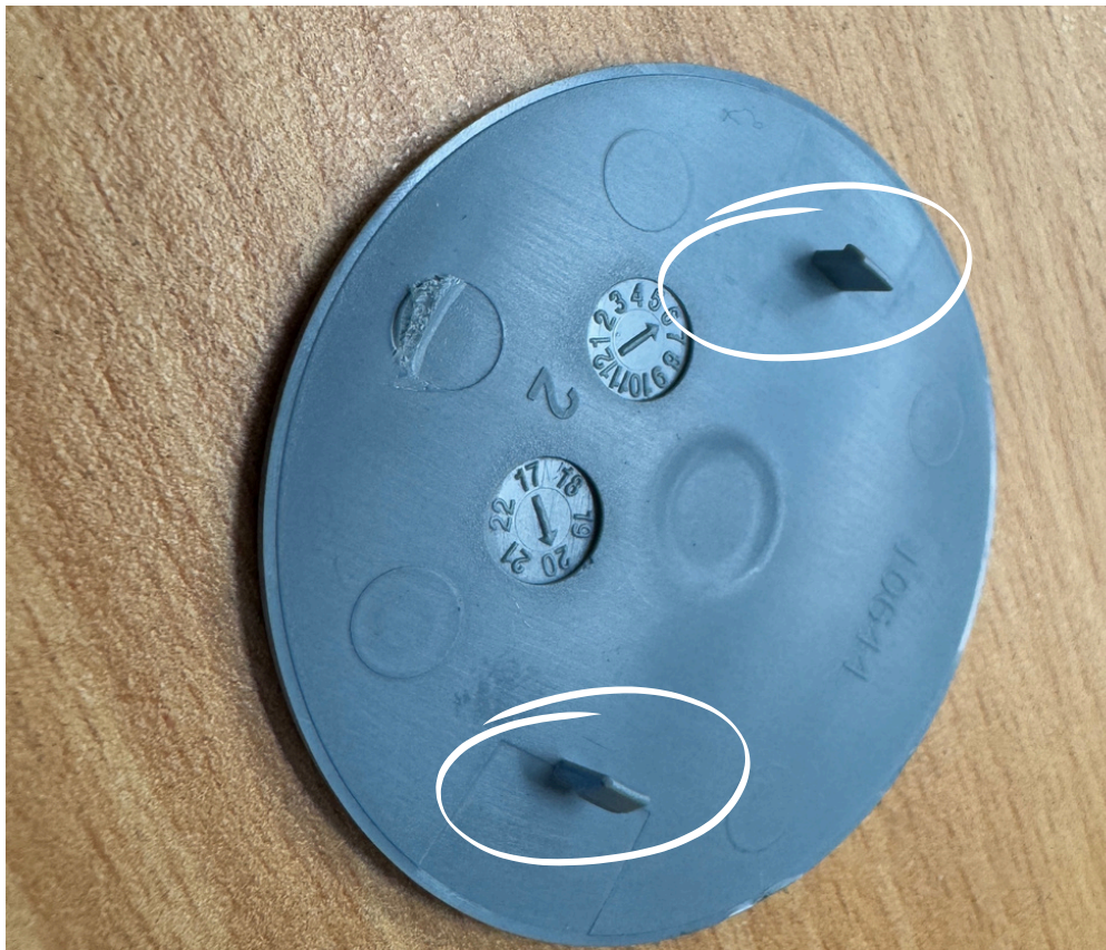
Rear wheel cover showing small clips that hold it in place
