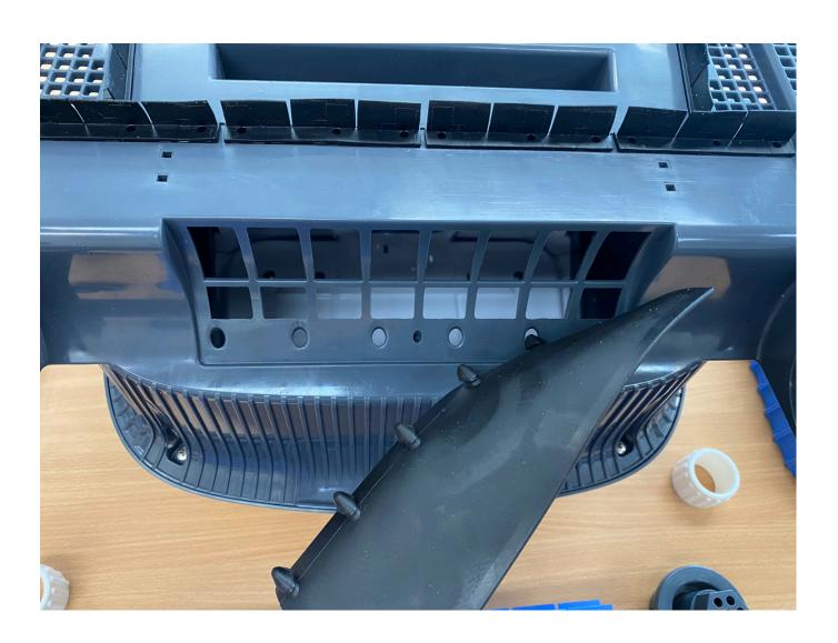
To ensure a tight fit, from the inside of the robot, use long nose pliers to pull the plugs in a little.
