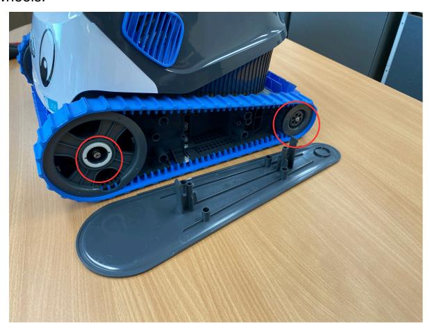
$\begin{array}{c} Step\ 2 \\ \text{Removing the screws will release the full track assembly} \end{array}$
