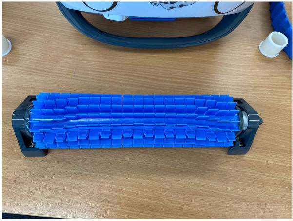
Replace the supplied parts, note that the active brush holder is not included in the tune up kit.
