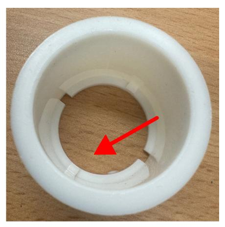
The above part is the front wheel bushing, there is one on each front wheel. Be sure to line up the lugs with the grooves on the chassis before tightening, failure to do so can crack the bushing. Rotate the bushing and you'll feel it locate to grooves.
