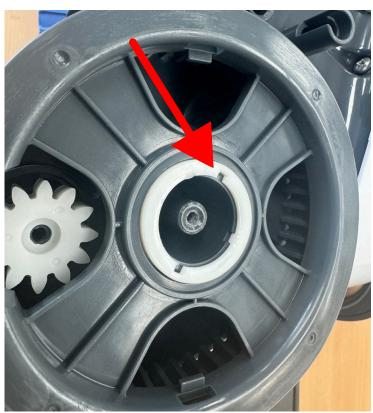
With the wheel bushing in place, slip the front wheel over the bushing. The small wheel disk and retaining screw then holds the wheel in place. Again be sure to line up the lugs on the disk with the grooves in the bushing before
