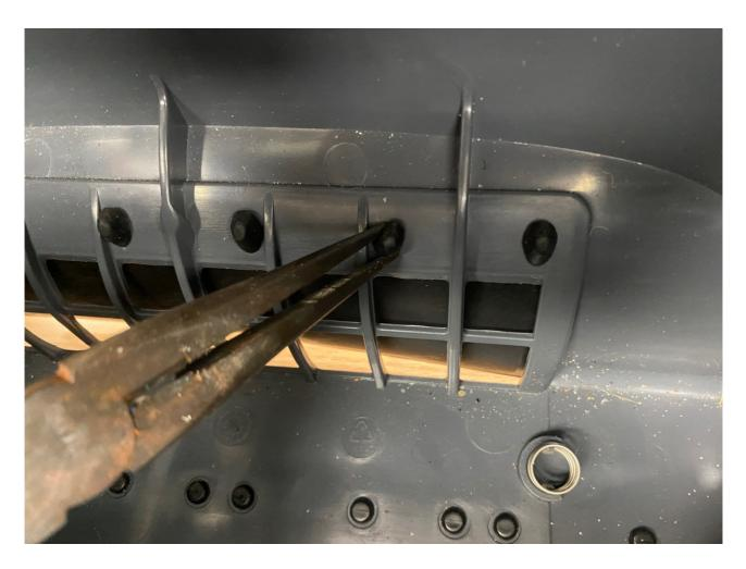
Once the Rapid Drain Flap has been installed you can go ahead and reinstall the front and rear brushes and tracks. Reinstall the side panels.
