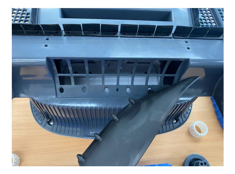
To ensure a tight fit, from the inside of the robot, use long nose pliers to pull the plugs in a little.
