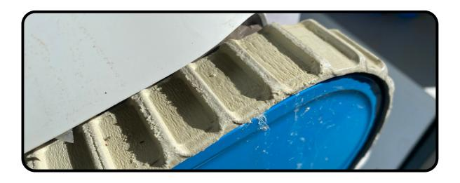
Decayed Tracks: When the rubber tracks of your robotic pool cleaner are subject to incorrect water balance they start to rapidly decay. This leads to them becoming soft and dissolving, when moving around the pool in this condition they will quickly fail. The tracks pictured are from an 18 month old robot that was subjected to 10+ chlorine levels.
