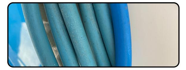
Discoloured Cable: In this image the cable that has been in the water is clearly discoloured when compared to the cable that has not entered the water.
