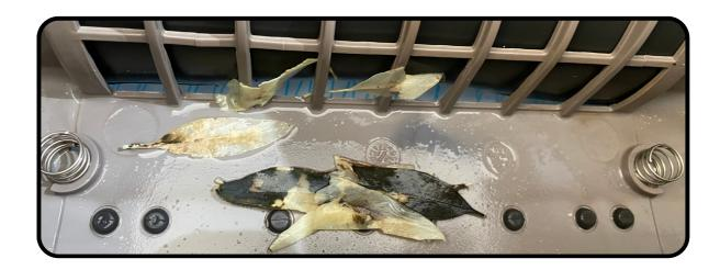
Bleached Debris: Shown here inside the filter chamber of a Maytronics S Series robotic pool cleaner are leaves that have been bleached white by the extreme chlorine levels. If you see bleached leaves in your filter basket, remove and rinse your robot imediately and then correct the problem.
