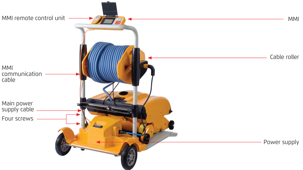
Figure 1: Assembling the Dolphin WAVE 200 XL - 1
